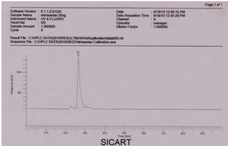
Figure 2: Chromatogram of standard Telmisartan solution (20 ng/ml)
