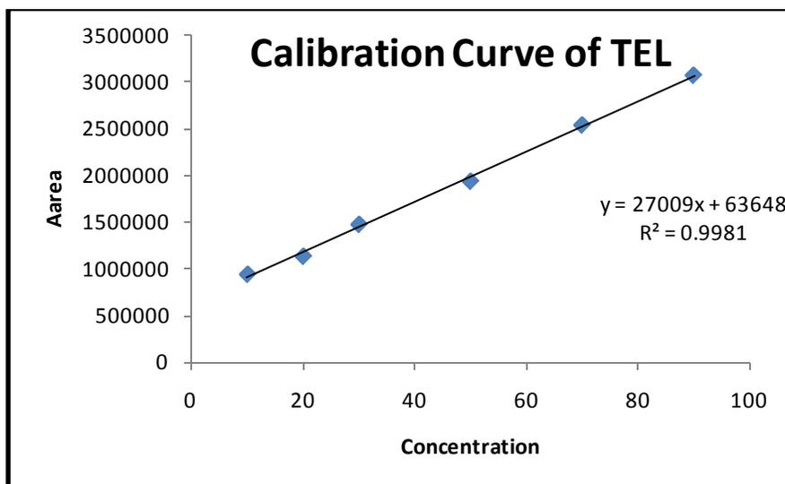
Figure 3: Calibration Curve of Telmisartan
